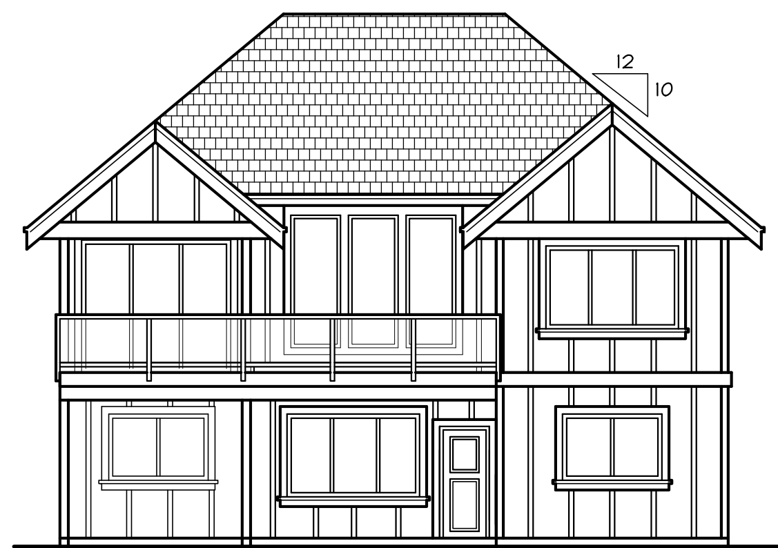
REAR ELEVATION 1/8" = 1'-0" NOTE: HOUSE TO HAVE A FIRE SUPPRESSION (SPRINKLER) SYSTEM INSTALLED PRIVACY FENCE NOT SHOW FOR CLARITY
